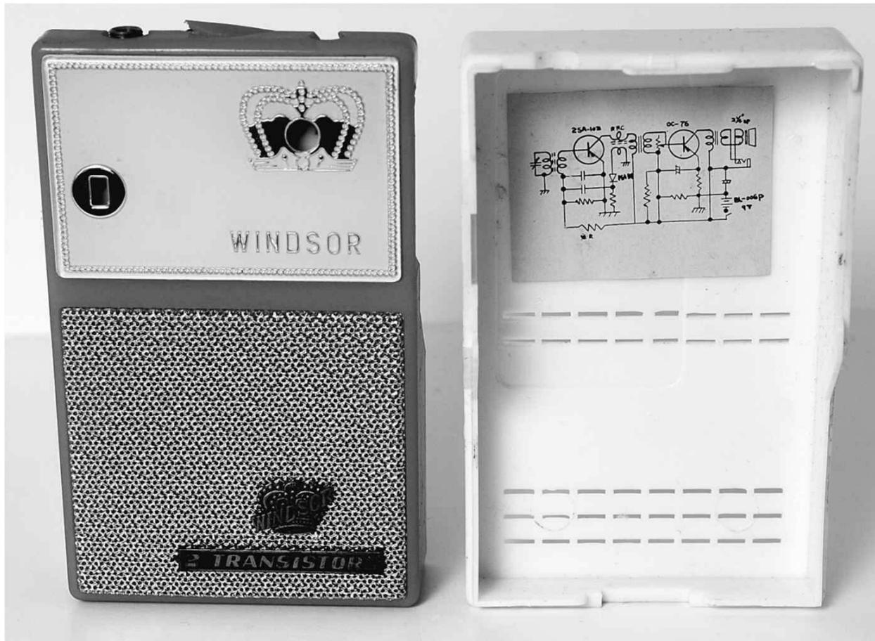
**Figure 6-1** Commercially made two-transistor reflex radio.
