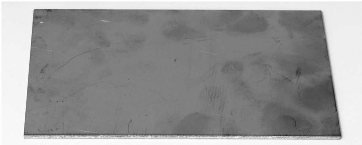
**FIGURE 3-23 Copper-clad board.**
