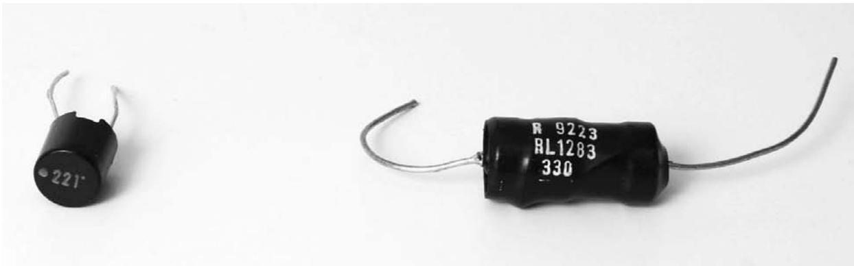
**FIGURE 3-13 Other inductors/coils.**
